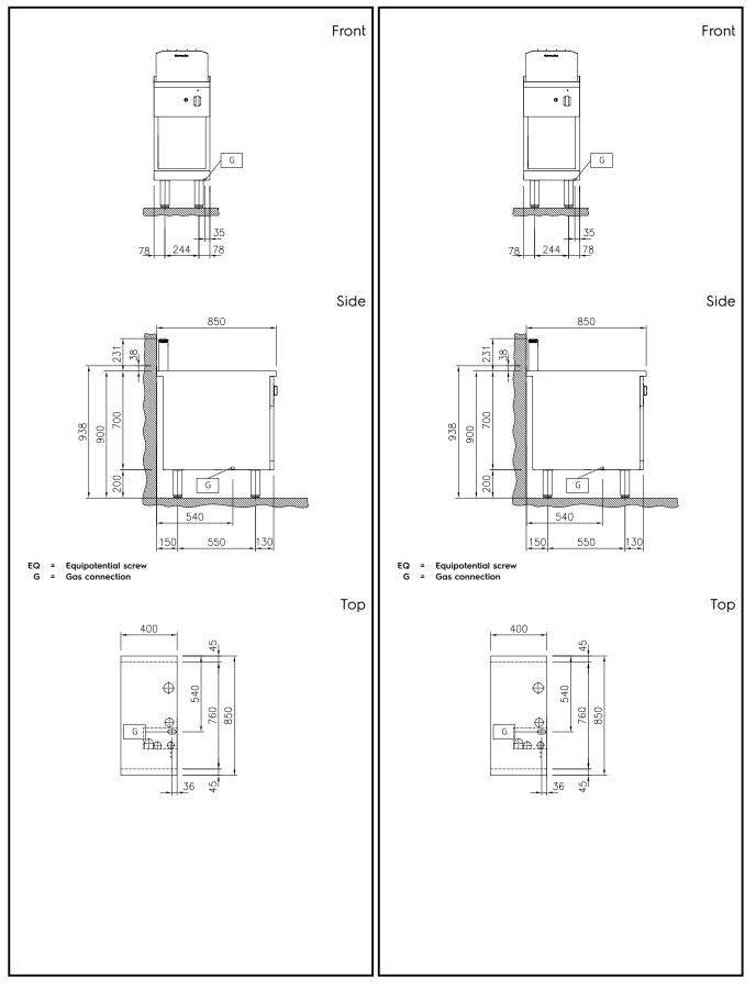
Modular Cooking Range Line thermaline 85 - Half Module Freestanding Gas Fry Top, 1 Side with Backsplash (Towm Gas) The company reserves the right to make modifications to the products without prior notice. All information correct at time of printing.
